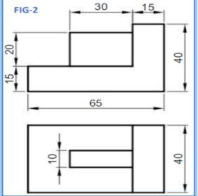
The front and side views of an angle plate are shown in above Fig. Draw its isometric view.
